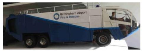
The cab side windows were tackled next and cut using the drawing I had made to mark and cut the body panels. These were heated and bent to conform to the cab sides and the black strips where the windows and doors open were cut from 1 x 1.5mm styrene strip and painted before
