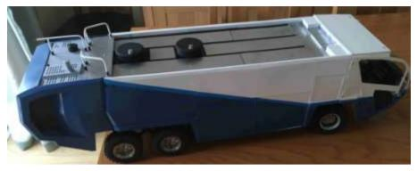
I next began to fabricate the plethora of safety rails using some styrene tube and  $16^{th}$  brass rod inserted to give the plastic some rigidity. And then turned my attention to the signage.
