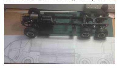
modify the Tamiya chassis so that the measurements were correct. This was achieved by simply moving the entire front axle assembly forward by 1cm.
