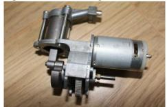
The motor and gearbox used is from a 12volt car tyre pump (left) as it gives the perfect 6:1 reduction needed to power the 6.8cm diameter four bladed brass propeller supplied in the kit. Originally I had intended to remove the the air pump side of the assembly but after experimenting with the smoke generator I discovered that the output of the pump could be utilised to accelerate the smoke on its way up the smoke stack.
