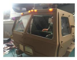
difficult because the windscreens are flush with the cab body and spent a lot of time cutting and forming the 1mm sheet acrylic to be an interference fit in the body. The side windows were a lot simpler as only the front part of the glass needed to be trimmed to a close fit as it has a sliding section rather like the early Mini cars
