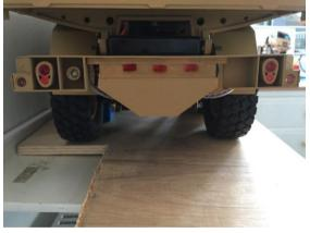
The rear lights are mounted on the rear bumper. If the truck bed lifts the bumper is fixed to the rear chassis member, if the bed is static the lights are fitted under the rear of the bed floor. I then made up the rear bumper bar adding, with a guess, the position of the lights from the various photos I have and after connecting all the lighting up tested that it functioned as intended.
