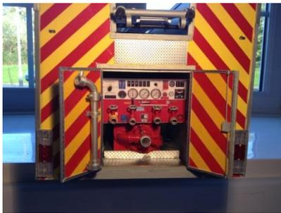
Using one of the photographs I had taken of the full size vehicle I copied and cropped the control panel and printed it the correct size before mounting it above the pump, then using some scrap styrene tube and Robbe 10mm hand wheels made up the outlet valves and fixed them to the lower part of the control board.
