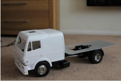
The cab had to be modified to add the rear 'crew' compartment and this was done by cutting the back off the moulding and inserting a scratch built section before replacing the back section. The aluminium base of the container section needed to be moved back and raised to allow room for the rear mudguards necessitating drilling and tapping new holes in the chassis and supplying four standoff spacers to raise the plate.
