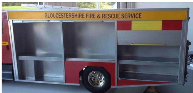
The empty lockers (left) have been populated by reference to the many photographs I took of the full size vehicles and all the items are scratch built. The many hoses that the lockers contain are made from turned aluminium tube ends connected together with red heat-shrink tubing and rolled to simulate the hoses in the full size vehicle.
