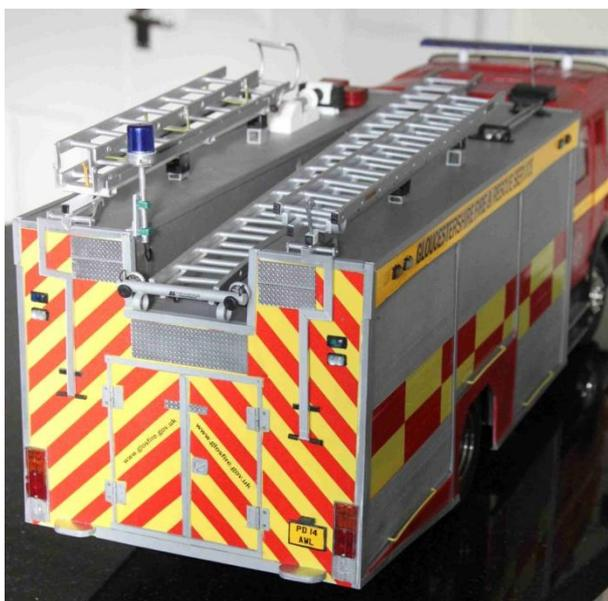
The blue lights at the front and rear along with the clear and amber lights over the roller shutter doors
