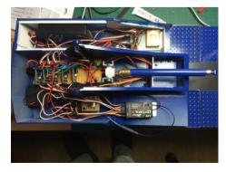
The rest of the top build went according to plan and after installing all the various esc's, receiver, switch system and sundry electronics into the crane body there was very little room for anything else. It looks a bit of a 'rat's nest' but is all functional. The only electronics outside of the crane section is the main drive ESC which is situated under the vehicle driver's seat.
