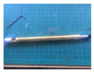
stainless steel threaded rod via an M3 captive nut, force fitted into the lower end of the stainless tube, which acts as the hydraulic piston. This worked well and could extend the tube right out to the end. Since then I have discovered that the huge load imposed on the tiny gearbox caused it to wear
