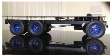
With the gearbox moved forwards I had to lengthen the prop shaft and utilised the existing dog drives set into the correct length of stainless steel tube. I then took some time to assemble the wheels after spraying them the nearest colour I could find to the actual vehicle (Fiat Capri Blue) I 3D printed the wheel hubs to cover the Tamiya fixing nuts and then turned to the next part of the build, applying the 2mm thick styrene build plate and fixing it to the chassis with brass standoffs.
