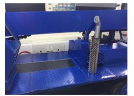
The board is accommodated in the centre of the truck between the chassis rails and under a removable section of the chequered plate that covers the whole top of the build plate.
