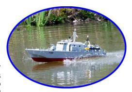
translated means Royal Ship the equivalent to our HMS. The boats were 96ft long with the main power being supplied by three, Rolls Royce marine Proteus, gas turbines driving through reverse/reduction vee-drive gearboxes to fully cavitating propellers and diesel engines providing the power for cruising and manoeuvring.
