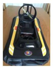
The kit supplied by Palaform contains a clear plastic screen to fit around the front of the open deck. Because of re-sighting the lift duct this required the inner part of the screen to be cut to clear it. Having done this I didn't like the finish and decided to spray the inside of the screen black to match the rest of the craft. In fact this enhances the overall appearance of the model considerably and after adding the yellow flashes that come with the kit I was very pleased with the result.
