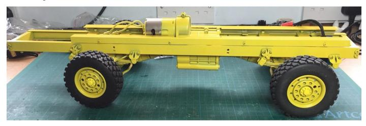
Some 10mm square styrene tube was placed on the top chassis members and fixed with internal cap head
