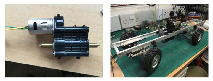
I now added the upper chassis members to achieve the correct height for the temporary build deck. The entire assembly was then broken down to give it a coat of grey etching primer and a top coat of yellow before being reassembled.
