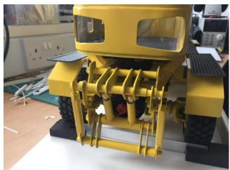
The next big issue was to fabricate the hydraulic assembly at the front which is used to attach the vehicle to the blower section. As this isn't shown on the Oshkosh drawing, I had to use some of the many photos I have of it to make the various working parts. I had to guess at some of it but in the end managed to produce quite a realistic version, made from styrene sheet and various tube sizes, that is operated by a servo mounted under the cab.
