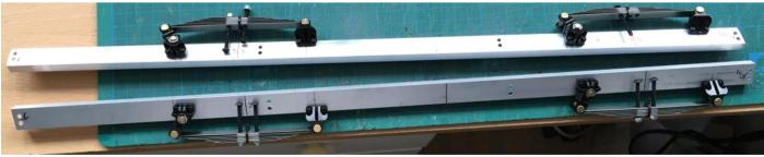
The cross members were made from stock aluminium bar machined at the ends to slot into the chassis sides and fixed using M3 x 6mm stainless cap head screws. Four lengths of the 15 x 10mm section channel were cut to form the fixing supports for the two metal geared servo's mounted over the axles and connected via 3mm brass rod and ball and socket style servo connectors.
