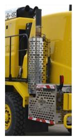
One of the difficulties I found was sourcing the staggered slotted sheet that surrounds the exhaust systems as shown in the image here. After many hours of fruitless searching on the internet I finally bit the bullet and decided to make my own. The sheets of 2 mm hole staggered aluminium I acquired for the vehicle walkways now
