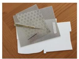
came in useful and after sandwiching a sheet of 0.5 mm styrene sheet between them I drilled through all the holes eventually producing a copy of the aluminium in styrene. From there it was just a case of using the scalpel to cut the plastic out between each pair of holes. A scrap piece of the finished item is shown on the image on the left.
