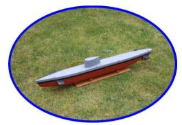
requiring only three channels, rudder, front planes and propulsion. The model was 30" long, made from 2mm liteply, designed as a simple dynamic diving submarine with fixed rear planes and controlled by the front planes for depth.
